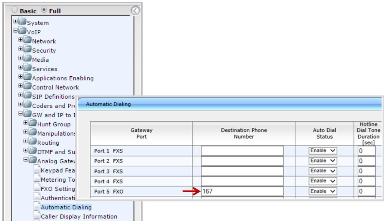
Figure 36: Configure automatic dialing rules for port 5
