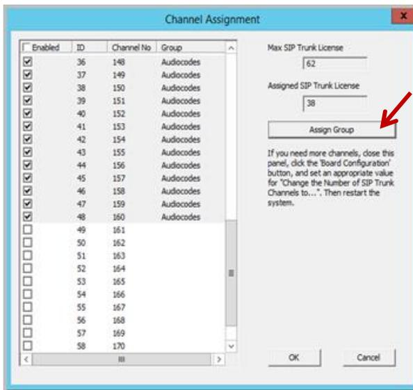
Figure 42: Enable channels
