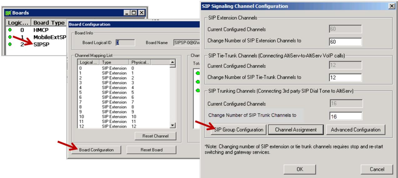
Figure 37: Open the SIP Group Configuration panel
