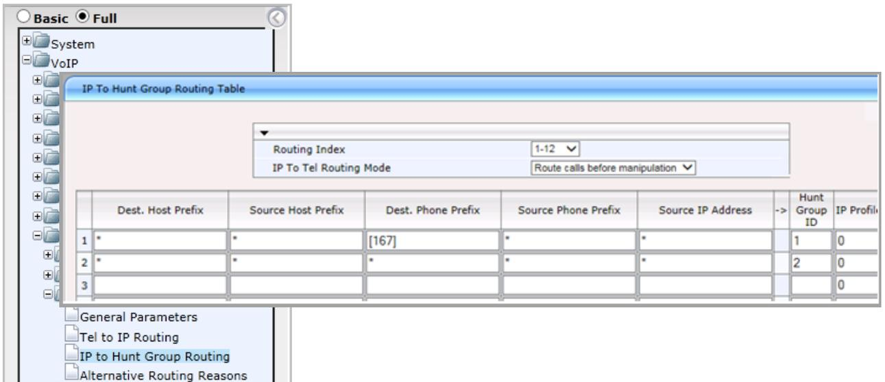
Figure 51: Configure IP to Hunt Group routing rules
