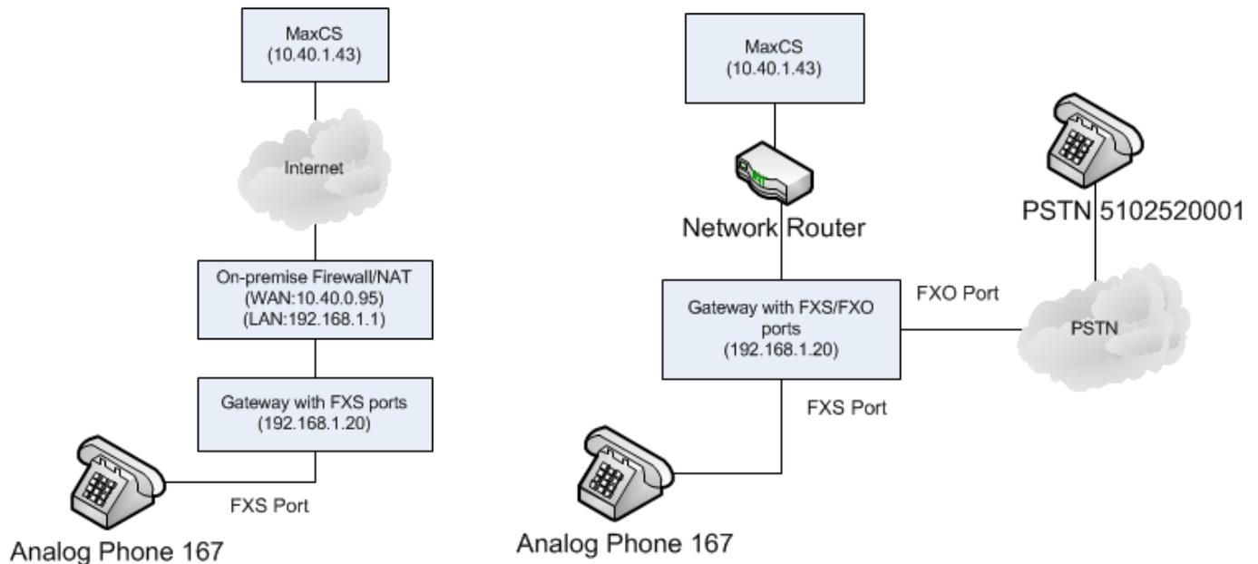
Figure 1: Example configurations for Internet and LAN deployments
