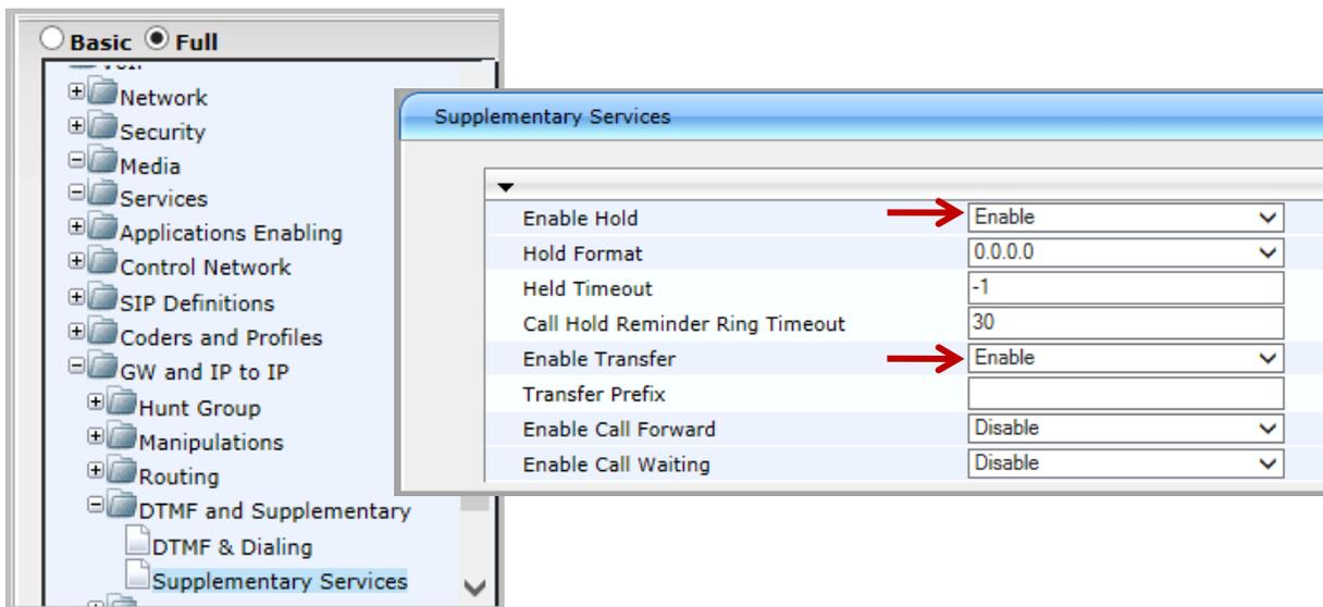
Figure 66: Adjust Supplementary Services parameters
