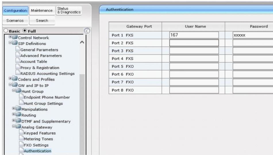
Figure 80: Re-entering the FXS extension authentication password if
