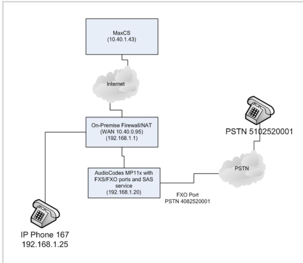
Figure 53: Architecture for Cloud environment
