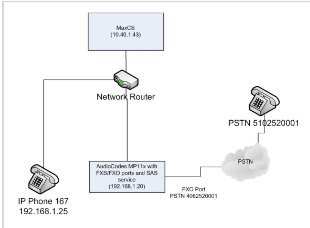
Figure 52: Architecture for LAN environment
