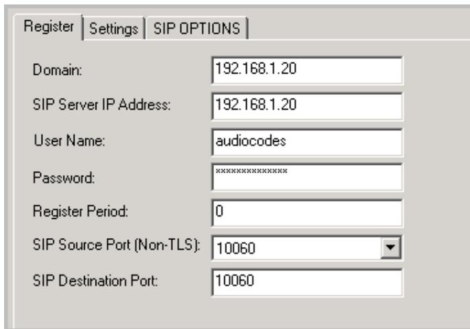
Figure 24: Configure the SIP server parameters
