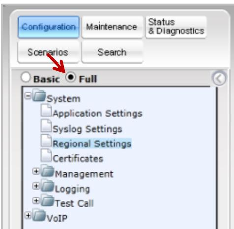
Figure 9: Set the AudioCodes tool menu to Full
