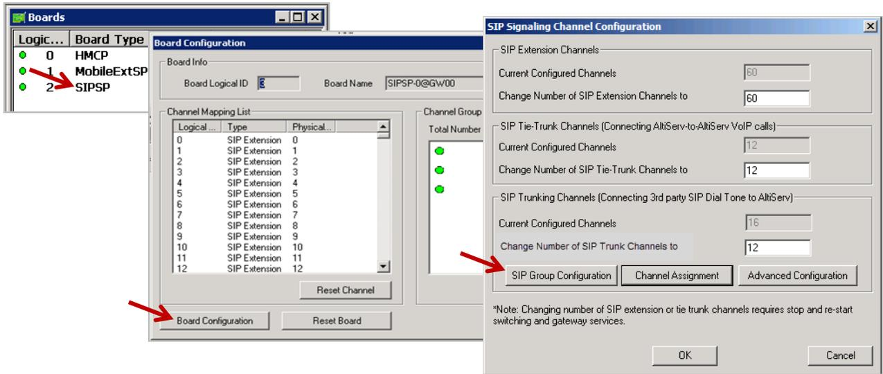
Figure 21: Open the SIP Group Configuration panel
