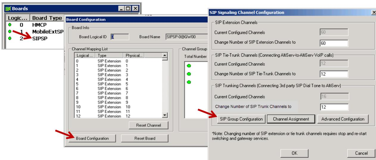
Figure 29: Open the SIP Group Configuration panel
