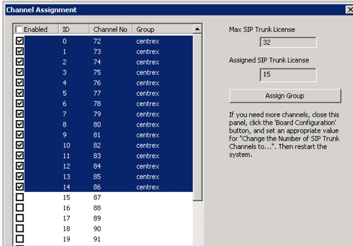
Figure 25: Enable channels
