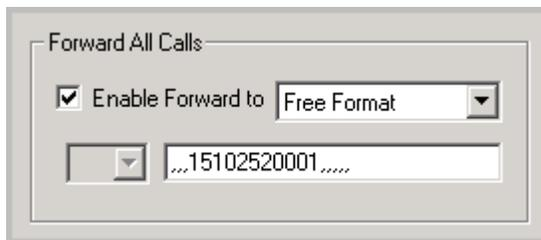
Figure 39: Insert commas to allow time for transfers to complete
