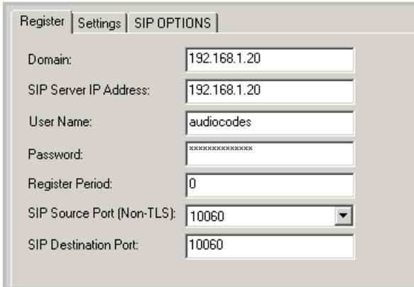
Figure 32: Configure the SIP server parameters
