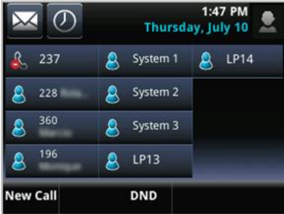
Figure 30: Example of a Polycom phone display showing Line Park slots LP13 and LP14
