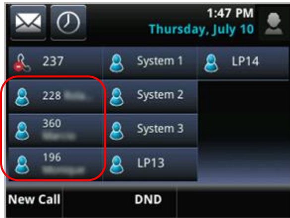
Figure 28: Example of a Polycom phone display showing BLF extensions on the left
