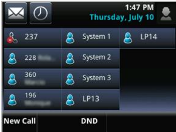
Figure 31: Example of a Polycom phone display showing Line Park slots LP13 and LP14
